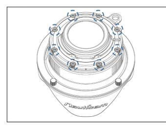
1. Remove the eight screws from the back of the lens.
