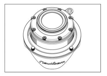
Secure the mounting ring by tightening the eight screws. Do not over-tighten, the screws only need to be snug.
