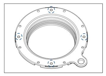
3. Observe the 4 small sockets in the bayonet ring. Place the bayonet ring onto the WWL and rotate the ring until it seats on the WWL.
